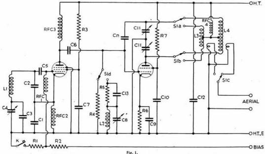
The oscillator stage of this transmitter is designed to minimise the effect of the valve upon the frequency. With great attention paid to mechanical rigidity and screening, and with LI constructed carefully and CI, C2, C3 and C4 chosen wisely, stability comparable with that of a crystal oscillator can be achieved. Component values are as follows:
