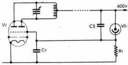
Series connection of stabiliser for good regulation of screen grid voltage with twin tetrode R.F. valve. Also applicable to single valves (807, etc.).
