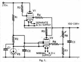
Constant voltage power supply unit. With 270 volts in from standard power unit, a sensibly constant voltage, variable at will between limits of approximately 100 and 230 volts, at any current up to 70 mA., is obtainable.
