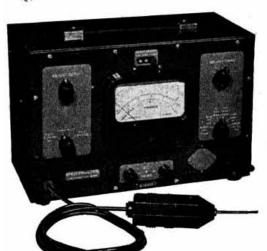
A highly stable D.C. Valve Voltmeter using an external diode probe for R.F. and A.C. measurements. Stability and freedom from zero drift are ensured by careful design and the simplified controls make for ease in handling. For A.C. mains operation, 110-120V and 200-250V, 40/100c/s.
