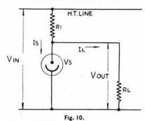
Basic circuit for deriving value of series resistor.
