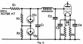
Screen grid stabilisation of 813, PT15 and similar high anode voltage valves. VS1 and VS2 can be Brimar VR150/30, giving 300 volts. R1 will be about 3,000 ohms, 5 watts.
