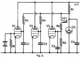
Stabilisation of exciter stages. All screens are connected to stabilised line.
